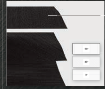
UD tape lamination The direction of the fiber in each layer of the tape lamination stack can be tailored to specific applications
