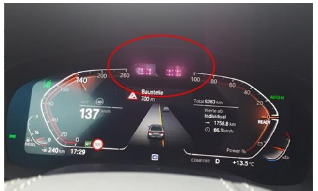
Glow in the dark effect of NIR LEDs captured with a cellphone camera, which is usually more sensitive than the human eye in the IR range.
