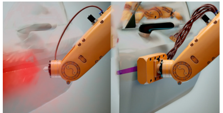
Traditional spray coating in automotive industry versus digital coating application.
