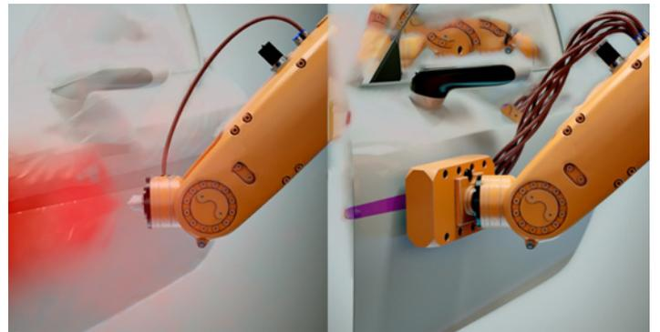
Traditional spray coating in automotive industry versus digital coating application.
